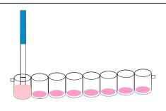
5. Insert the "Immersed" end of the strip into the mixture; Incubate for 5 min at room temperature again.
