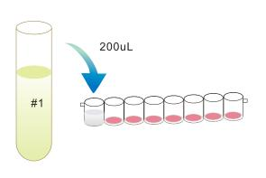
3. Take 200ul sample into the wells using pipet. You can also then put the well into the well holder to avoid sample spill.
